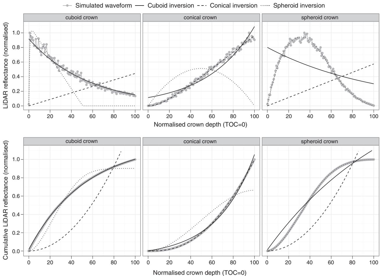
**Fig. 4.** Testing of the analytical expressions against simulated waveforms for archetype crowns (cuboid, conical, spheroid) with LAI 4 with no prior information of tree and crown height (experiment 2). Crown depth ranges from 0 (top of crown) to 100 (bottom of crown). (upper row) Analysis of the original waveform; (lower row) Analysis of the cumulative waveform.
